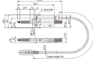
\* Upon installation, clamp the stem. Unit: mm
