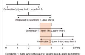
In measurements where judgment output GO (OK) signal and comparator combinations (4 sets) are observed in PLC I/O, four sets of comparators are switched from the 1st set to the 4th in turn and a comparator for which judgment output becomes GO has an OK region. (If judgment output becomes GO in the 3rd set, the comparator concerned has the region of 3 mm or more to 4 mm inclusive.)
