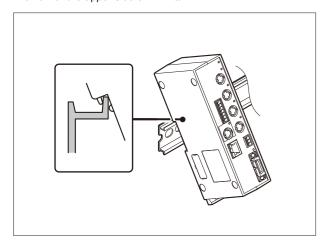
Push and install the MG41 main unit until a click is heard so that the lower side of groove on the back of the MG41 main unit is fit into the DIN rail.
