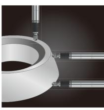
Tapered roller bearing measurement
