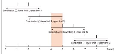
Example 2: Case where the counter is used as a 9-stage comparator
