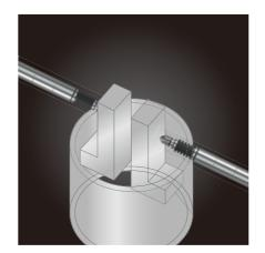
Bearing inner diameter measurement
