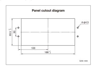
Reference: If a mounting screw hole cannot be drilled in the panel, the MG43 may be installed using four screws on the back of the main unit.
