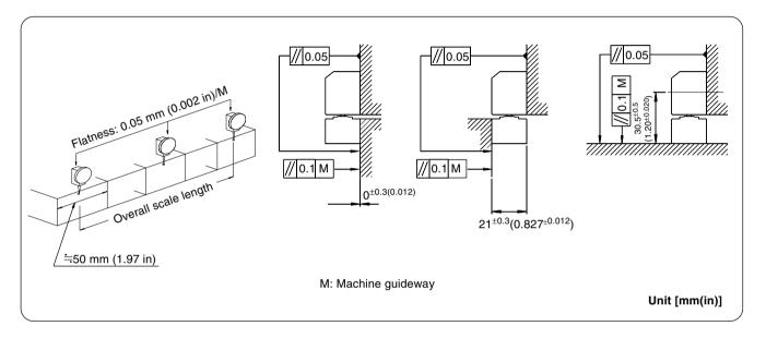
• Design the installation surface so that the parallelism of the installation surface and the scale in the vicinity of each scale mounting screw is 0.05 mm (0.002 in).
