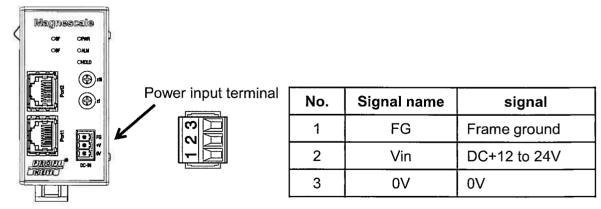
\*The power supply of the module connected to MG80-CM is supplied from MG80-EC. Supply power is 2.4W plus the total power of the connected module is required.
