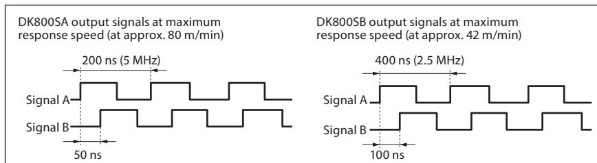
This measuring unit outputs AB quadrature signal with a maximum frequency of 5 MHz and minimum phase difference of 50 ns for the DK800SA, and a maximum frequency of 2.5 MHz and minimum phase difference of 100 ns for the DK800SB. Use a counter or controller that can process these signals.
