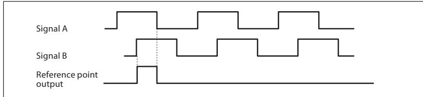
The reference point is the synchronized reference point that is at Hi level when the signal A and signal B are at the Hi level.
