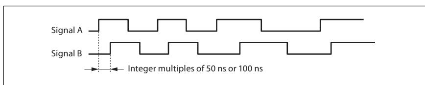
In the standard specifications, the minimum phase difference is fixed at 50 ns for the DK800SA and 100 ns for the DK800SB, but the minimum phase differences in the table below are available as custom specifications.
