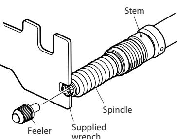
Fig. 2 Attaching/removing feeler
