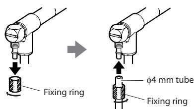
Fig. 6 Attaching the  $\phi 4$  mm tube
