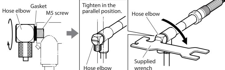
Fig. 5 Attaching the hose elbow
