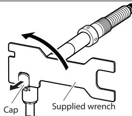
Fig. 4 Removing the cap
