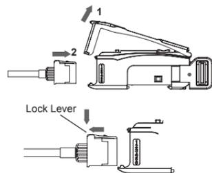
To remove it, press and hold the lock lever then pull the measuring unit out.
