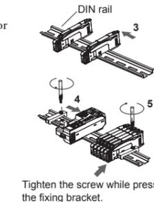
For the maximum number of modules that can be connected, refer to the specifications of counter module. Always use the fixing brackets.
