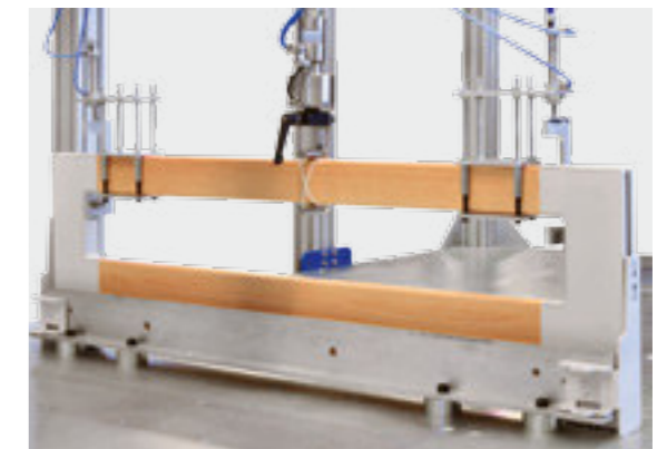
Test of side rails on nursing care beds in the universal test field
