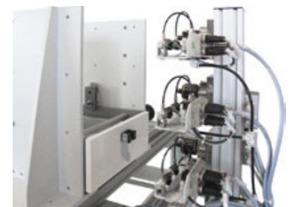
Test rig for max. three drawers
