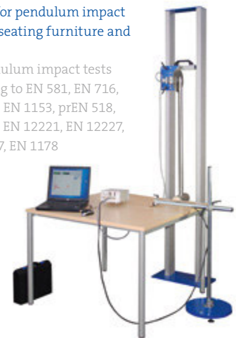
Test rig for pendulum impact tests
