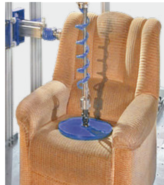
Armchair testing in the universal test field
