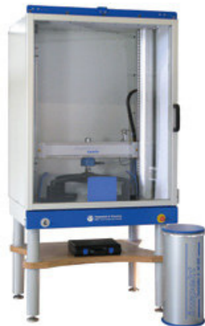
Universal testing machine, amongst others, for testing star bases according to BIFMA X5.1
