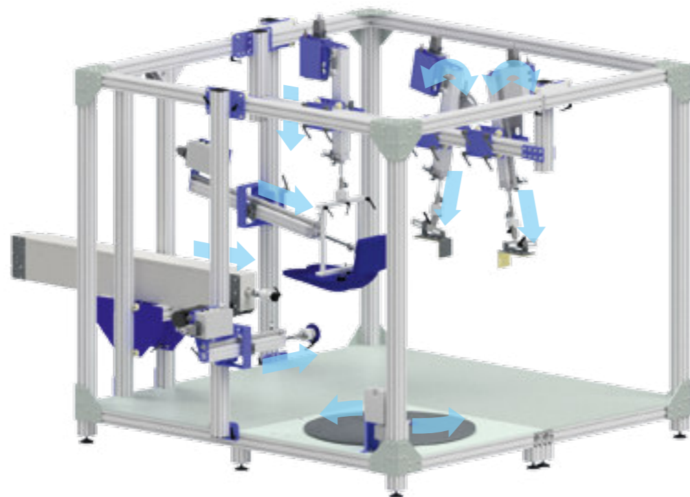
Demonstration of possible movement and load directions of the test axes in a universal test field
