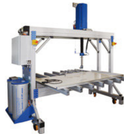
Test rig for 90° peel tests on solar modules
