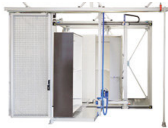
Test rig for cabinet doors and drawers
